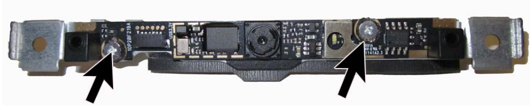
Figure 6-44 Disconnecting the webcam module cable
